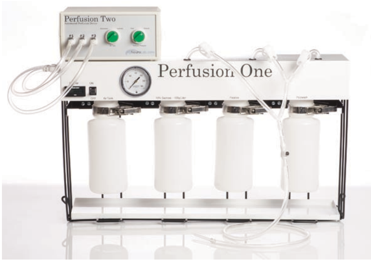
Fig. 9.1 Perfusion Two™ apparatus for sacrifice perfusion. The bottle on the left serves as an air pressure tank, the next bottle is prewash solution, then fixative. The 4th bottle is optional for a postwash if desired
