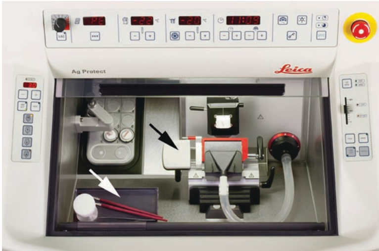
Fig. 4.7 Leica 1950 cryostat; one of several versatile inside views. The black arrow shows a hand rest for brush users. The white arrow points to the embedding shelf. The tube is connected to the vacuum antiroll devise on the stage which also doubles as a vacuum cleaning device for the cryostat
