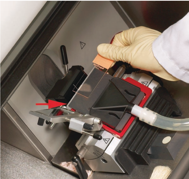
Fig. 1.8 The figure shows a tissue section being retrieved from the cryostat stage. The antiroll mechanism has been reflected to the left. The red arrow points to the blade clamped in the blade holder. The operator must be aware of the proximity of their hand to the blade at all times to avoid injury when retrieving sections
