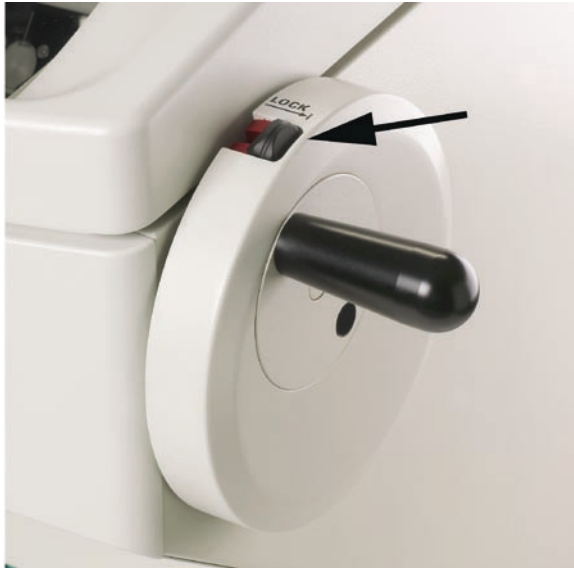
Fig. 1.6 Cryostat handwheel. Each turn of the wheel advances the tissue block the precise increment of section thickness setting. The arrow indicates the locking mechanism
