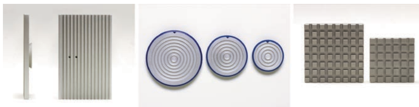
Fig. 1.4 Specimen holders or chucks. Specimen holder of different sizes and shapes are made to accommodate various embedding tasks
