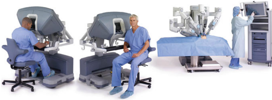
Fig. 9.13 The complete da Vinci Si System with dual surgical consoles offered as a optional capability
