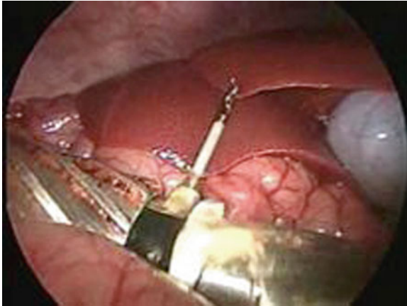
Fig. 6.2 Mobile biopsy robot performing liver biopsy as viewed from laparoscope. (With kind permission from Springer Science+Business Media: [42])
