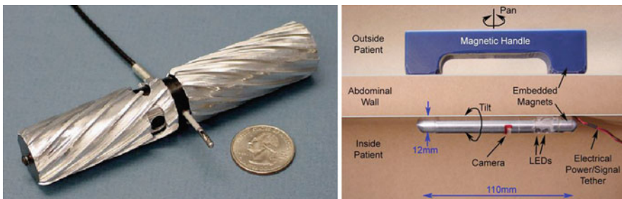
Fig. 6.1 Mobile ( left ) (© 2006 IEEE) and peritoneum-mounted ( right ) imaging robots [36, 40]
