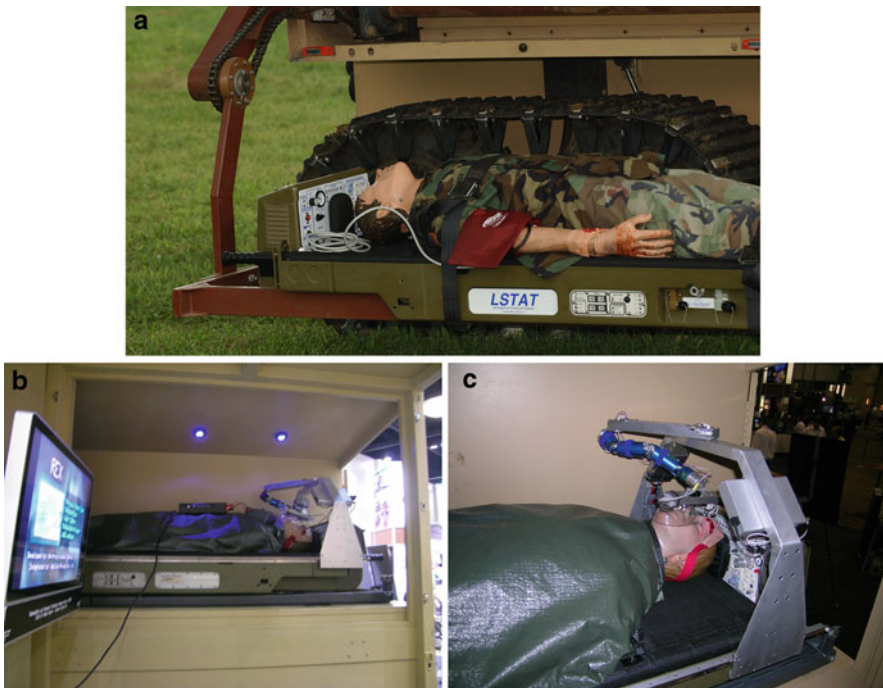
Fig. 2.5 Life support for trauma and transport (L-STAT): (a) integrated with REV; (b) L-STAT mounted in TAGS-CX patient transport pod;(c) L-STAT with Carnegie Mellon University serpentine robotic arm casualty assessment prototype
