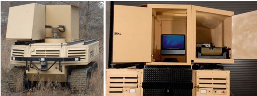
Fig. 2.2 Tactical amphibious ground system – common experimental ( left ); CX with patient transport & attendant modules ( Right )
