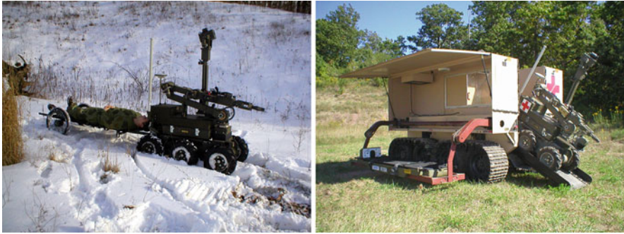
Fig. 2.1 Robotic extraction (REX) and Robotic evacuation vehicle (REV) prototypes ( left ); REX towing casualty on litter in snow ( right )
