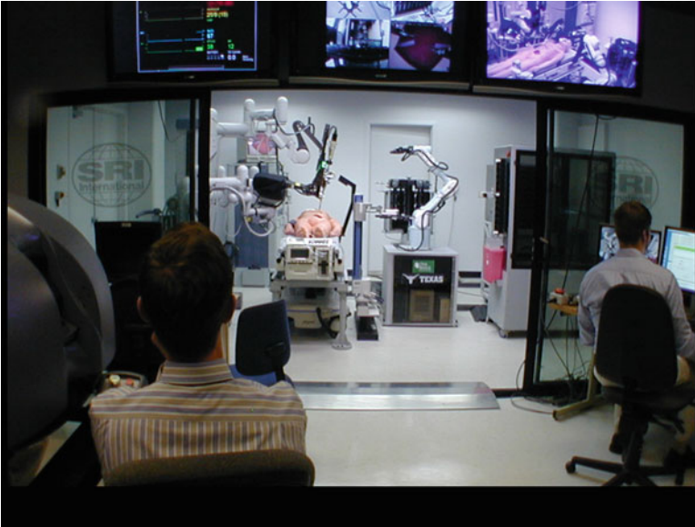
Fig. 1.2 Prototype 'surgical robotic cell' – the 'operating room without people' (Courtesy of Pablo Garcia, SRI International, Menlo Park, CA 2008)
