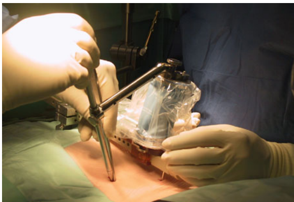
Fig. 11.2 SpineAssist assembly in a less invasive pedicle screw insertion. A guiding tube attached to the robot arm guides the surgical tool along a predefined trajectory
