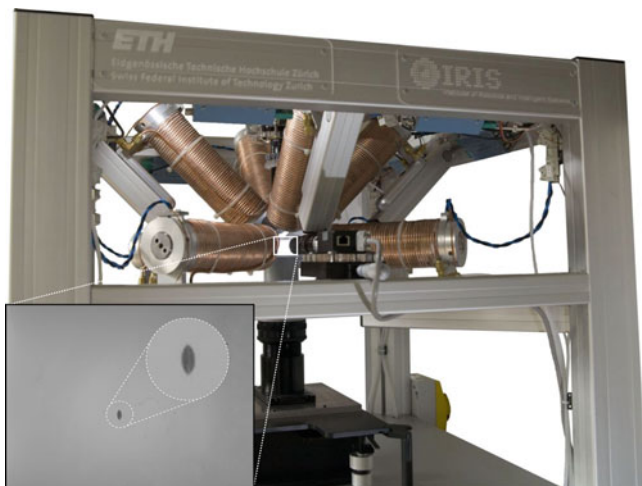
Fig. 13.14 OctoMag prototype: The system contains eight 210-mm-long by 62-mm-diameter electromagnets (©IEEE 2010), reprinted with permission. The gap between two opposing electromagnets on the lower set is 130 mm. The inset shows a 500- \mu\text{m} -long microrobot of the type described in [66] levitating in a chamber. This is the side-camera view seen by the operator
