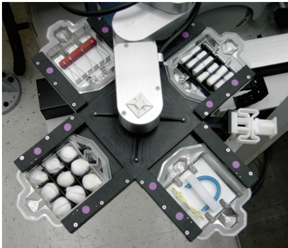
Fig. 3.22 Four supply trays, each held by a capture mechanism with three purple fiducial marks, in the fast cache
