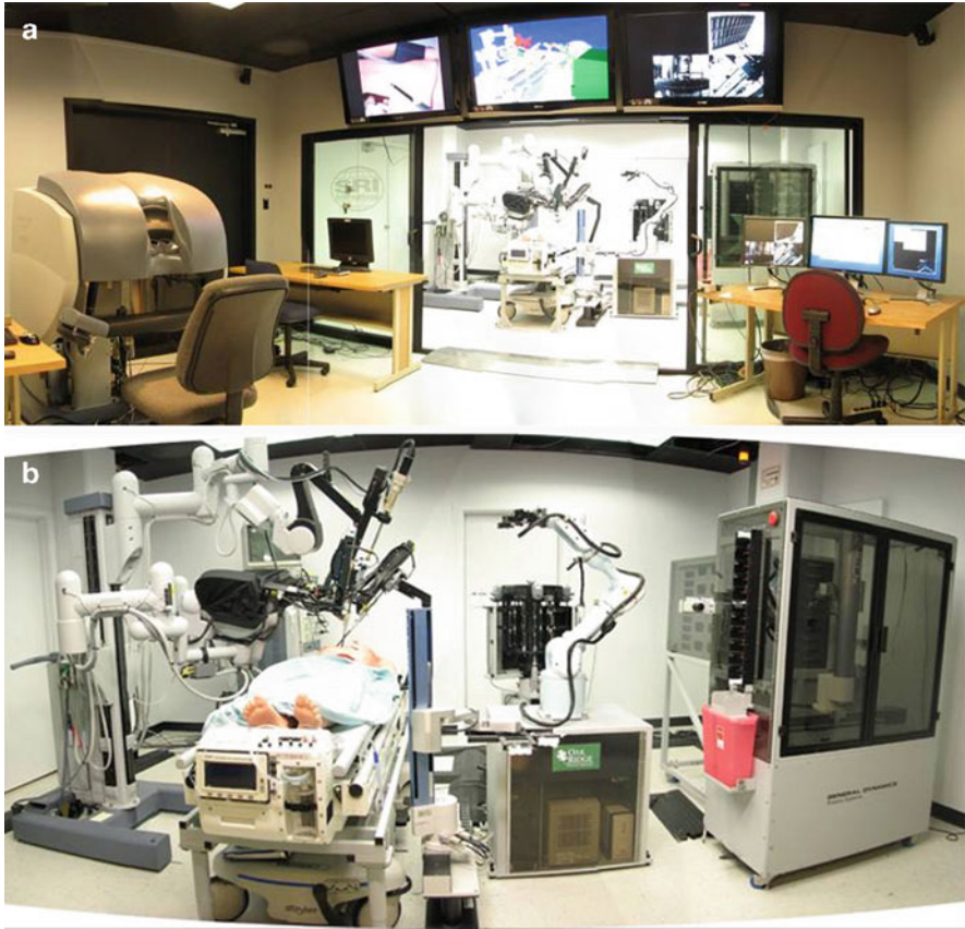
Fig. 3.8 The TP system (a) control cell (b) surgical cell
