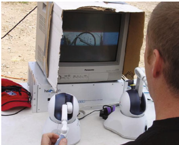
Fig. 4.3 Surgeon manipulating the RAVEN remotely in the high desert of Simi Valley, California
