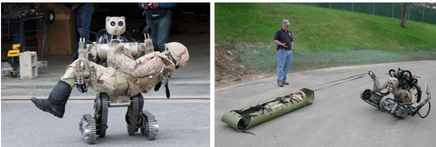
Fig. 2.3 Battlefield extraction assist robot (BEAR) prototype ( left ); BEAR extracting casualty with foldable litter ( right )
