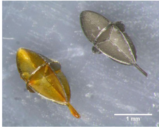
Fig. 13.2 Microrobot utilizing a functional coating (©IEEE 2008), reprinted with permission. Right: A bare magnetic microrobot made of thin assembled nickel pieces, based on [66]. Left: A microrobot coated with an oxygen-sensitive film
