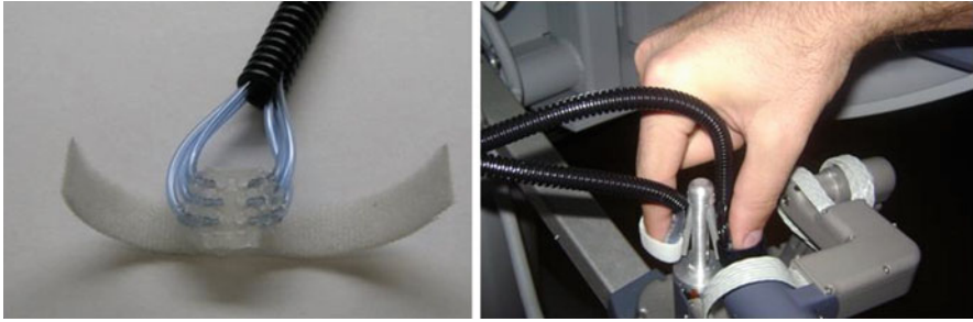
Fig. 19.2 Actuator array ( left ) and mounting on the da Vinci master controls ( right ). (© 2008 IEEE), reprinted with permission
