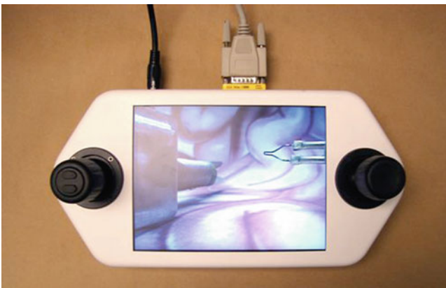
Fig. 6.7 User interface for dexterous manipulator robot. (With kind permission from Springer Science+Business Media: [41])
