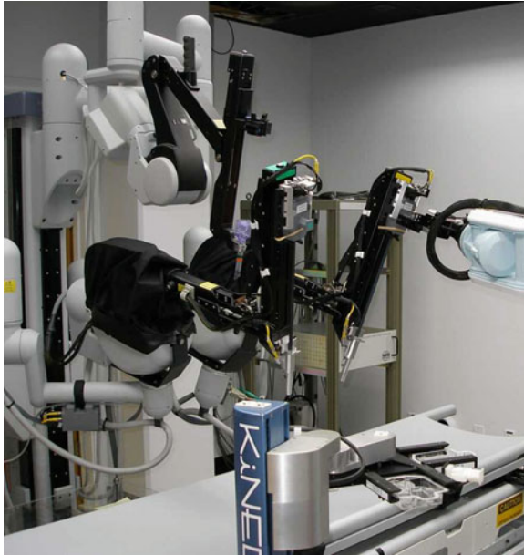
Fig. 3.11 Tool autoloader subsystem (TAS) mounted on each da Vinci arm
