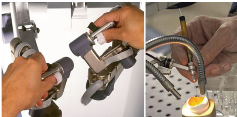
Fig. 18.5 A da Vinci master interface ( left , ©2010 Intuitive Surgical, Inc.) and a Steady-Hand Robot ( right , credit: Will Kirk, Johns Hopkins University) are representative of impedance-type and admittance-type master interfaces, respectively
