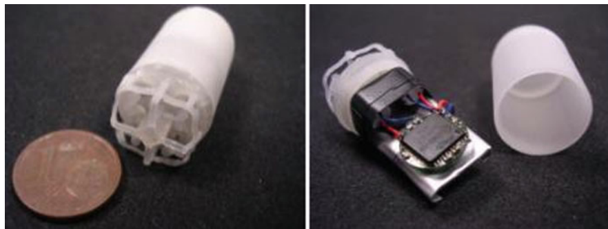
Fig. 14.13 Assembled capsule ( left ); view of the internal components ( right ) (© 2009 Taylor & Francis) [15]
