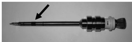
Fig. 31.3 Robot trocar. The thick black band denotes the remote center of the robot ( arrow ), the pivot point at which the robotic arm rotates in space
