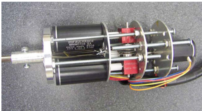
Fig. 7.10 Actuation motors and reduction mechanisms at head of instrument
