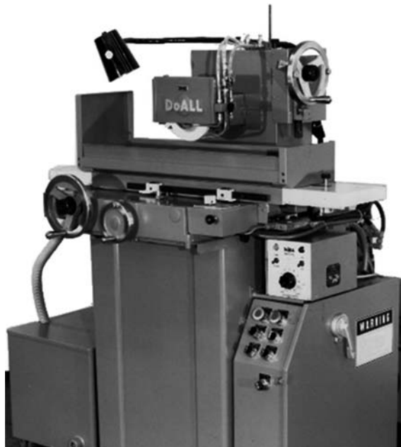
Fig. 1.11 The surface grinder is commonly used to finish flat surfaces (DoAll Co.)
