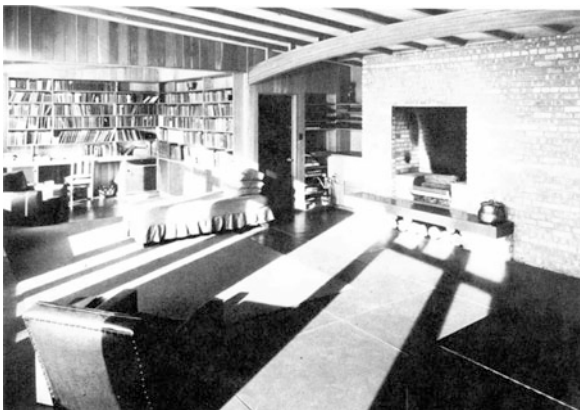
Passive Solar Heating in Built Environment. Figure 5 Direct gain maximized in the Duncan House (picture by permission of Pilkington, North America, Inc.)
