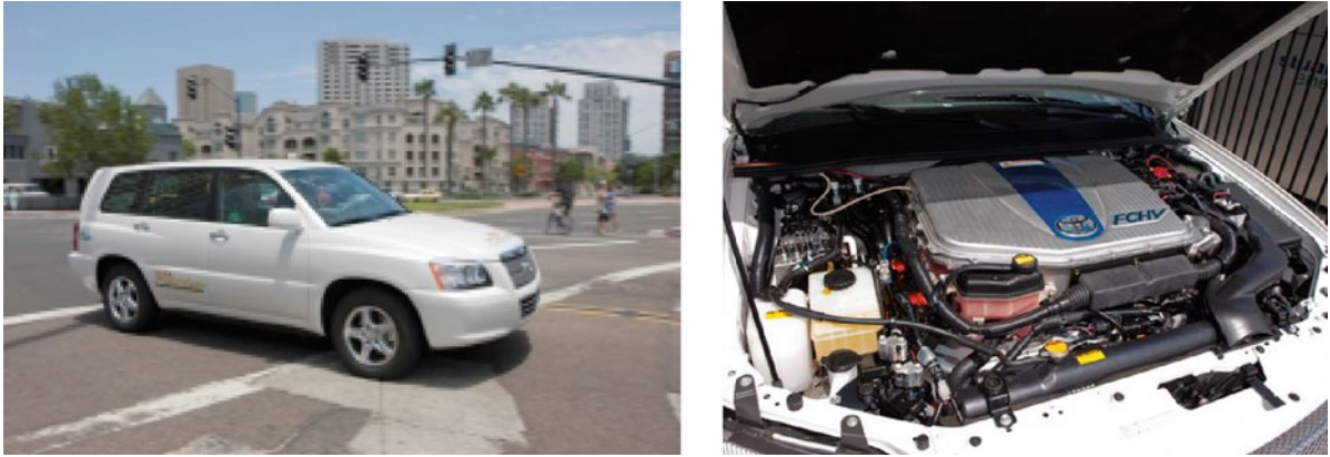
Polymer Electrolyte Membrane (PEM) Fuel Cells, Automotive Applications. Figure 6 Images of Toyota's FCHV-adv installed with their PEMFC stack [29]
