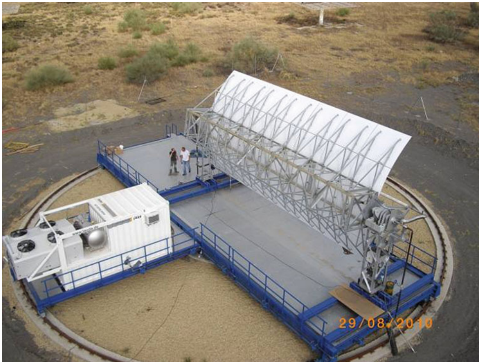
Parabolic Trough Solar Technology. Figure 10 Parabolic trough test platform at Plataforma Solar de Almería, Spain
