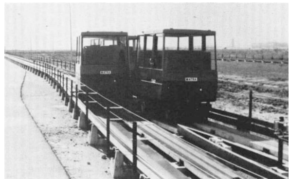
Personal Rapid Transit and Its Development. Figure 8 Aramis vehicle, France (Reproduced from [11]. With permission)
