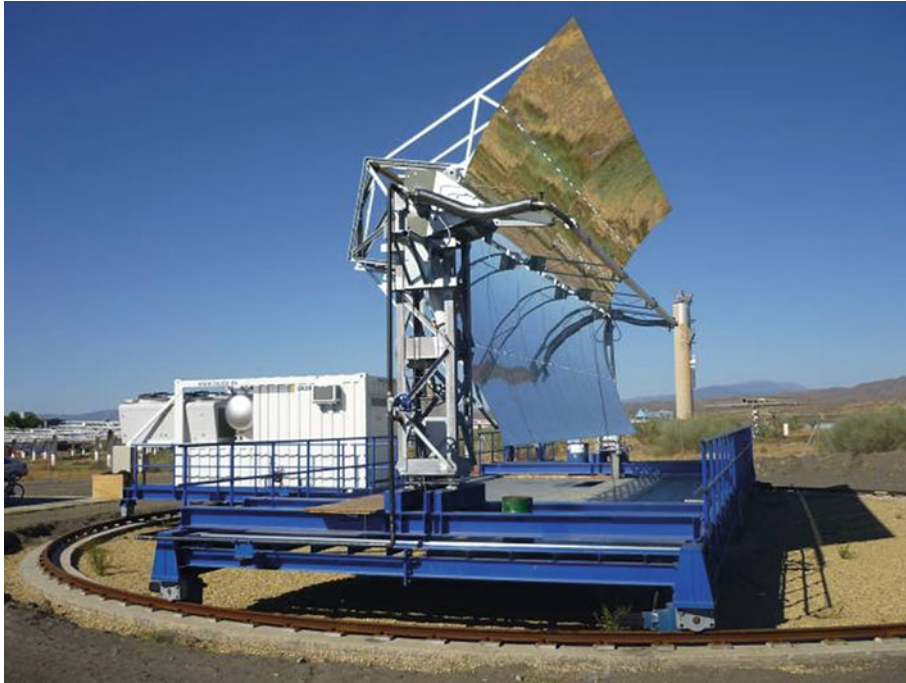
Parabolic Trough Solar Technology. Figure 11 Parabolic trough test platform at PSA, Almería, Spain
