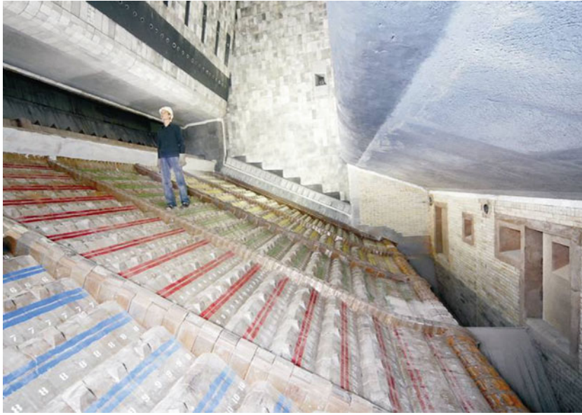
Martin Waste-to-Energy Technology. Figure 6 Reverse-acting grate
