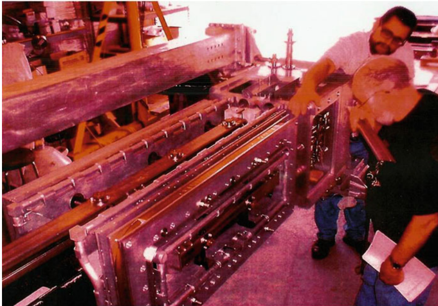
MAGLEV Technology Development. Figure 46 Assembly of Maglev-2000 superconducting quadrupole
