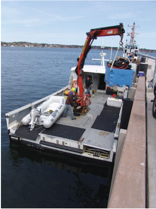
Mussel Culture, Open Ocean Innovations. Figure 4 A hydraulic articulating crane on a service vessel, shown here being used to unload equipment, is used extensively in mussel farming operations
