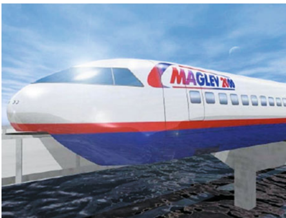
MAGLEV Technology Development. Figure 39 Artist's drawing of Maglev-2000 vehicle on monorail guideway
