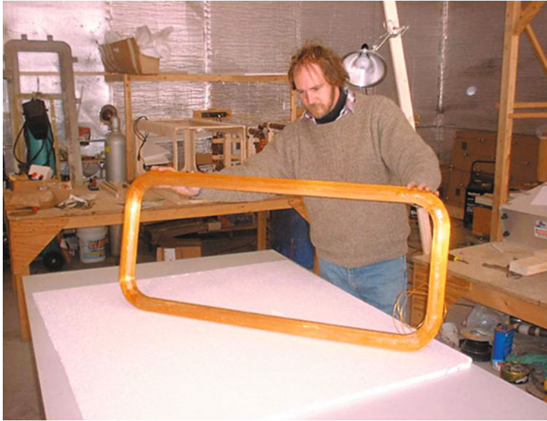
MAGLEV Technology Development. Figure 43 NbTi superconductor loop for Maglev-2000 quadrupole
