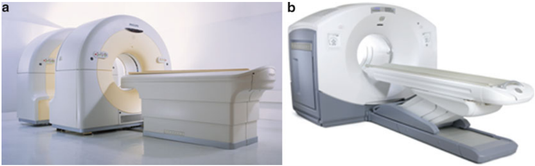
Fig. 3.4 Open PET/CT scanner design from Philips Medical Systems (a) compared with a conventional closed system (b). The conventional design shown is for the GE Healthcare Discovery 600
