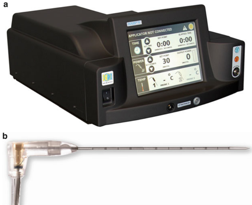
Fig. 11.11 Microsulis microwave ablation. (a) The 2.45-GHz Sulis V system powers a single MWA antenna. The control panel allows the user to set and monitor ablation duration and power. The bottom row of the panel shows temperature readouts from up to two separate 18-G thermal sensors that can be placed adjacent to ablation volume for added feedback on tissue status (Images courtesy Microsulis Medical Ltd., Hampshire, UK)
