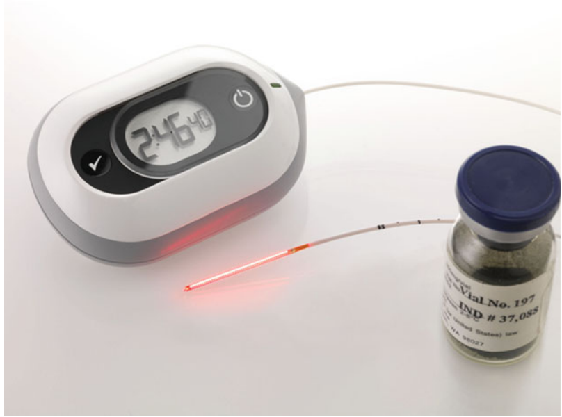
Fig. 11.17 Life Science Oncology. A small power/supply with clock is shown wired to the 1.2-mm-diameter array of LEDs ( red light ). The latter is placed interstitially, and treatment is effected by activation of intravenously injected Aptocine (vial) by the light (Image courtesy Light Sciences Oncology, Bellevue, WA)
