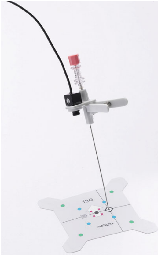
Fig. 7.2 The ActiSight (ActiViews, Haifa Israel) navigation positioning is determined by mapping the 2D coordinates of the colored reference markers in the camera image to the coordinates of the radio-opaque prints of the same markers in the 3D computed tomography images
