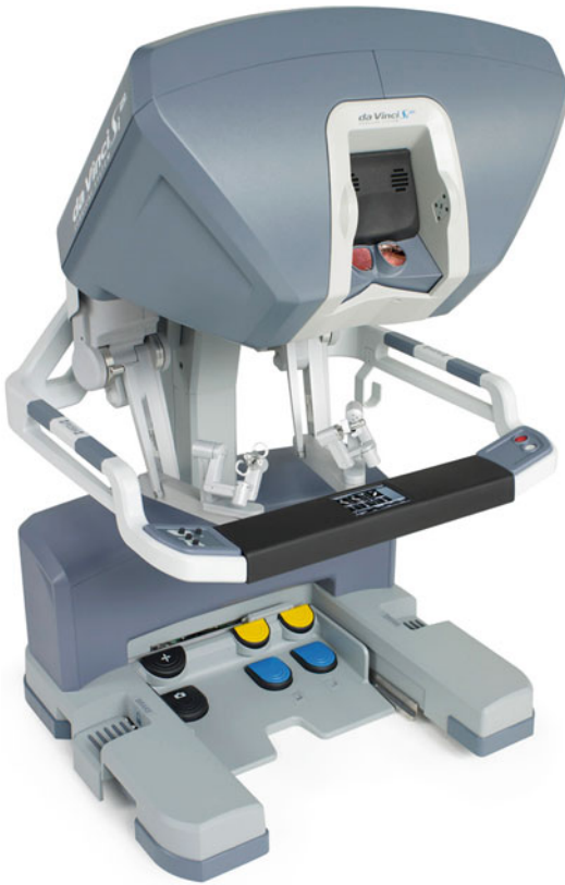
Fig. 52.7 da Vinci Surgical System Console, Intuitive Surgical®. This console allows the surgeon to have a 3-dimensional magnified view of the surgical field and to perform the dissection by controlling the robotic arms with enhanced dexterity, motion scaling and tremor reduction, 7 degrees of freedom, and 90 degrees of articulation (© 2010 Intuitive Surgical, Inc.)
