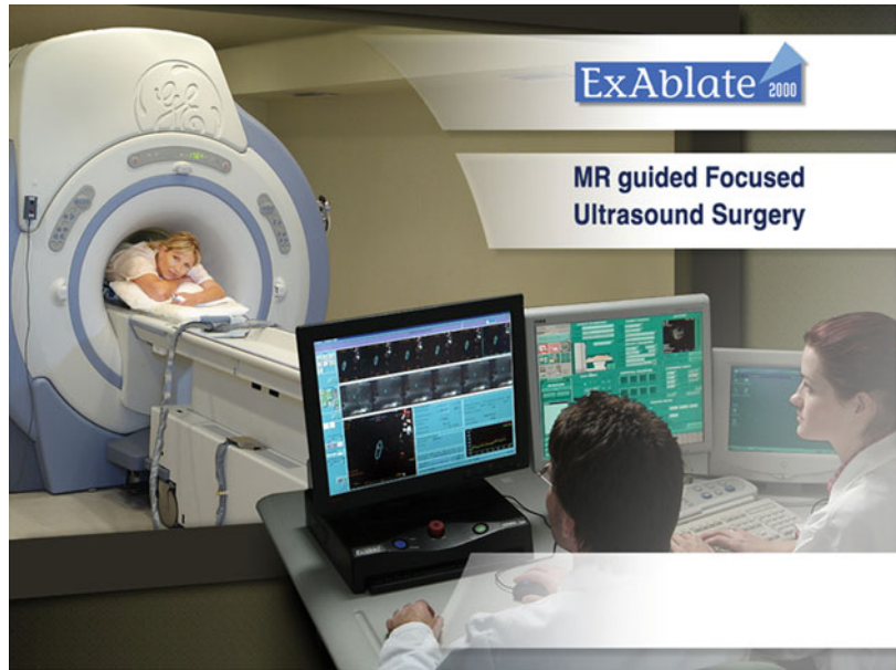
Fig. 36.1 Image of patient in MR scanner about to undergo MR-guided focused ultrasound. This patient is about to receive FUS as a treatment for uterine fibroids. Note the modified MR table which contains the MR-compatible focused ultrasound. The patient in this case is lying facedown so that the anterior abdominal wall is opposed to the water bath which contains the transducer (Courtesy of InSightec, Ltd.)
