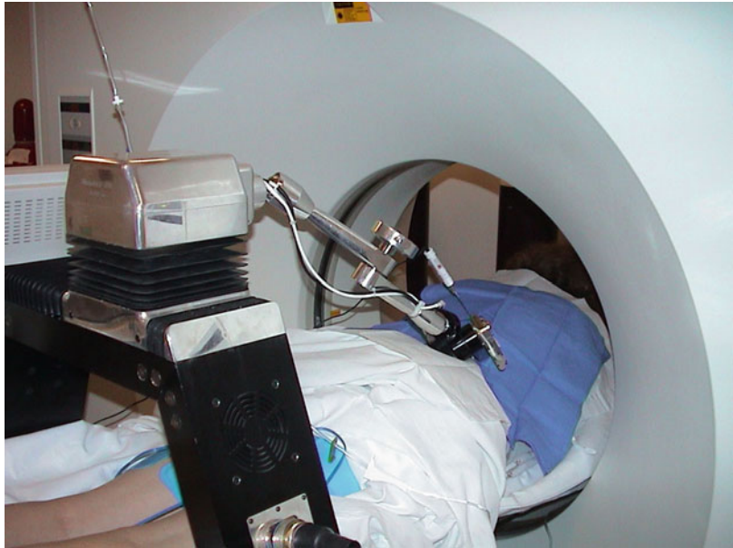
Fig. 17.5 Depicts the AcuBot which is a CT robot for needle placement. The robot is mounted to the CT table and can be registered with the CT image
