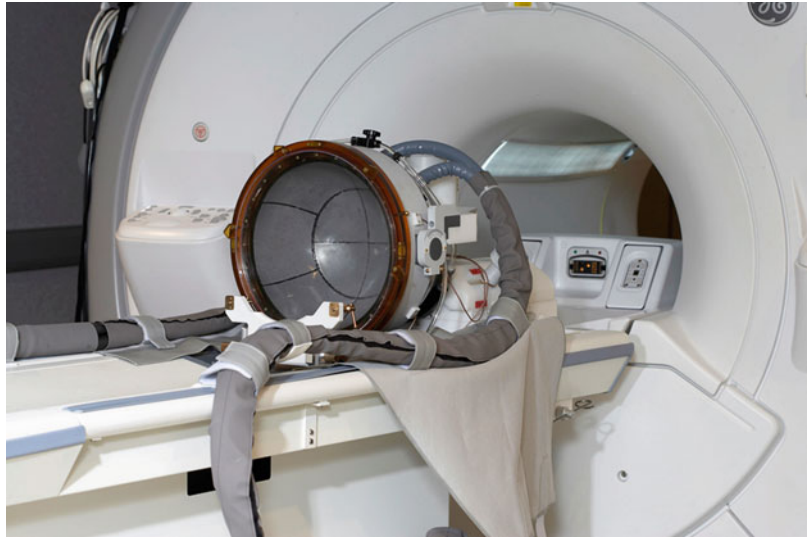
Fig. 5.10 A clinical prototype brain treatment system (ExAblate 3000, InSightec, Inc., Haifa, Israel)
