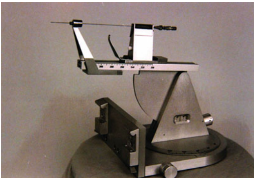
Fig. 59.2 Stereotactic module with a mounted biopsy needle – manually operated
