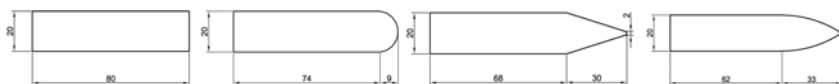
Fig. 11.2 Geometry and dimensions (in mm) for blunt, hemispherical, conical and ogival nosed projectiles [5] [10].
