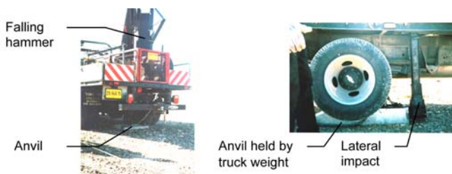
Fig. 17.8 Refraction survey: pressure waves (left) and shear waves (right).
