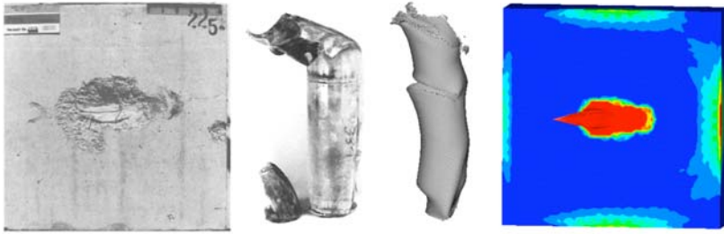
Fig. 9.8 200m/s impact footprint and deformed penetrator after a limit Ricochet chase in simulation and experiments at WTD91 and EMI.
