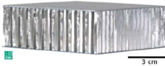
Fig. 21.2 Generic Honeycomb Sandwich Panel with Aluminum Facesheets.
