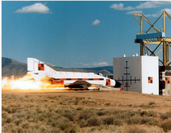
Fig. 16.13 The instantaneous photograph of the F-4 impacting the target (Courtesy of Sandia National Laboratories).
