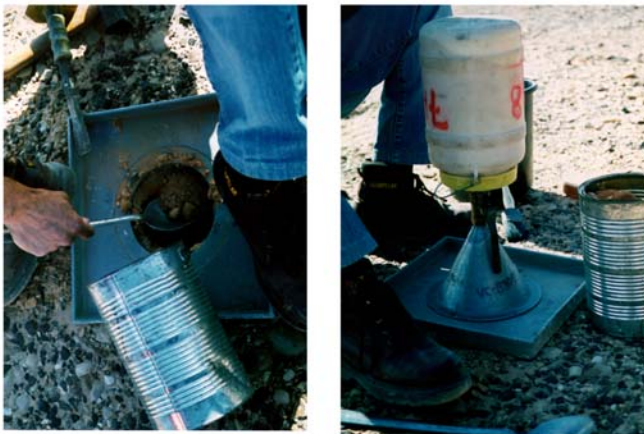
Fig. 17.7 Sampling field density (Sand Cone): sampling (left) and hole volume measurement using a given density sand (right).
