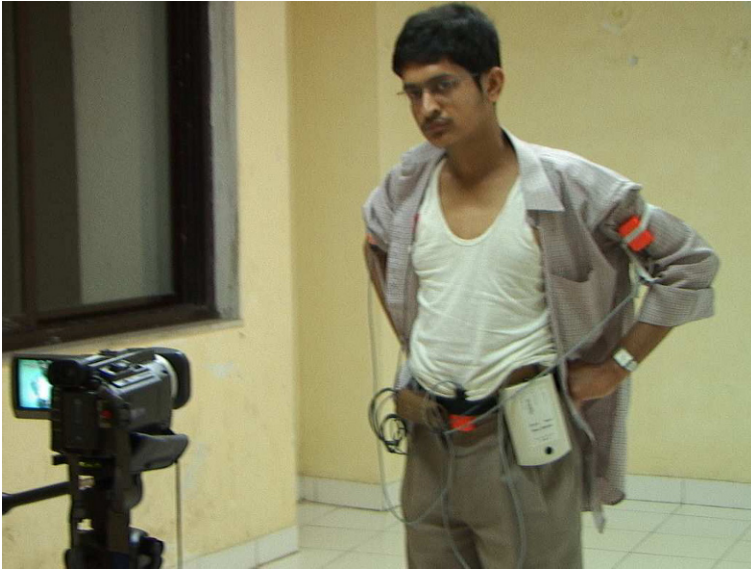
Fig. 5.1. Illustration of the experimental setup. Motion trackers (small orange objects) are strapped on the upper arms and the waist. The bigger object hanging at the waist where the left hand touches is the bluetooth interface for motion sensors. The single lead ECG recorder is attached to the front right side of the waist. The entire experiment is recorded on video to capture stray events not recorded by the motion sensor.
