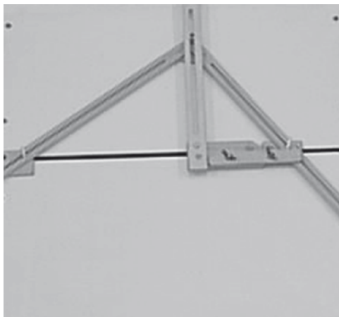
Fig. 11.6 Cavalieri's tool to draw an arc of parabola
