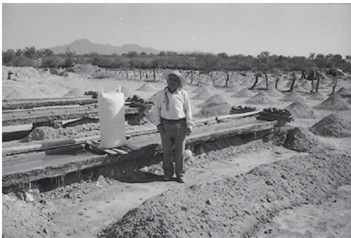
Fig. 2 Salt producer in Simirao (Lake Cuitzeo Basin, Michoacán) standing in front of his canoas, or wooden troughs, used in the solar evaporation of the brine. Note the sack of crystallized salt on the canoa, and the little mounds of prepared soil (used for leaching) all around the finca, or salt-producing unit
