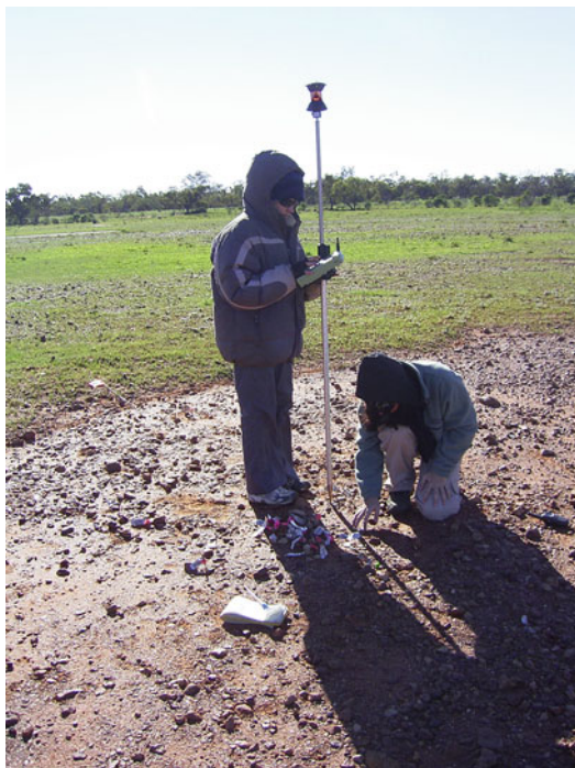
Surface Survey: Method and Strategies, Fig. 1 Self-tracking total stations allow the rapid location of artifacts in three dimensions. Colored nails are used to mark stone artifacts
