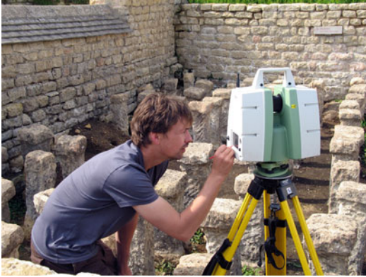
Buildings, Archaeological Study of, Fig. 2 Laser scanning carried out by the University of Birmingham at Chedworth Roman Villa, Gloucestershire (UK), on behalf of the National Trust (Photo: Jason Wood)
