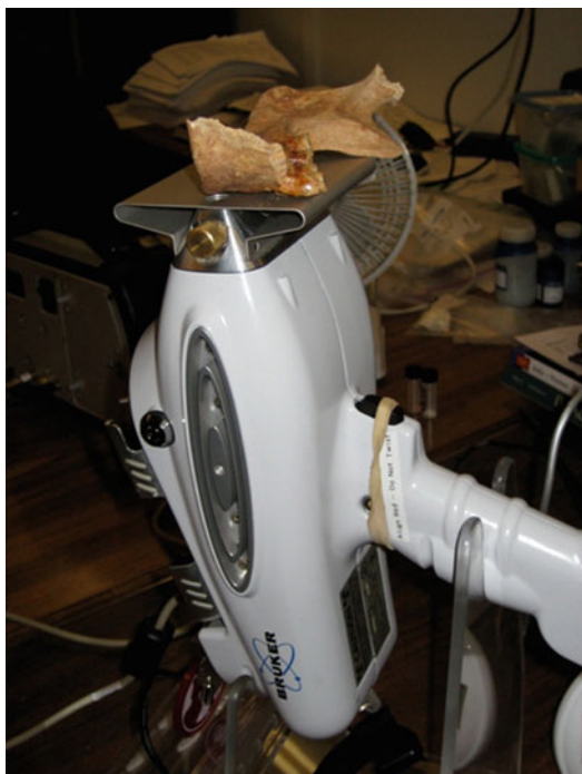
Bone Chemistry and Ancient Diet, Fig. 7 Nondestructive trace element analysis of bone using a portable X-ray fluorescence spectrometer
