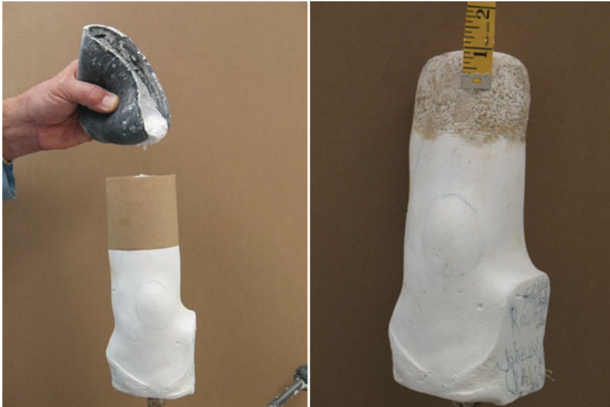
Fig. 20 Method to adjust the depth of the socket. A trouble free approach is simply to add plaster to the end of the cast that is used as the mold to produce the socket ( Left panel ). The end of the cast can be built up at least 1 in. or 25 mm ( Right panel )
