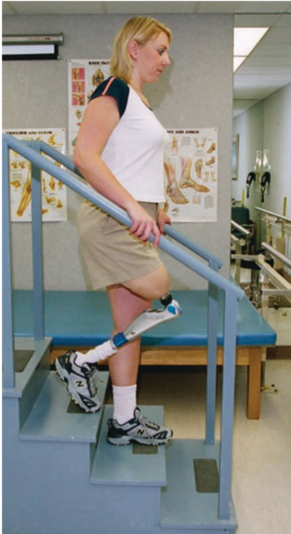
Fig. 18 Microprocessor knee. Regulates swing and stance resistance facilitating ability to descend steps
