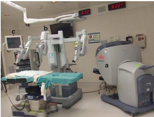
FIG. 31.1. Displays (a) the console (b) a three arm da Vinci® robot surgical system and (c) video monitor.
