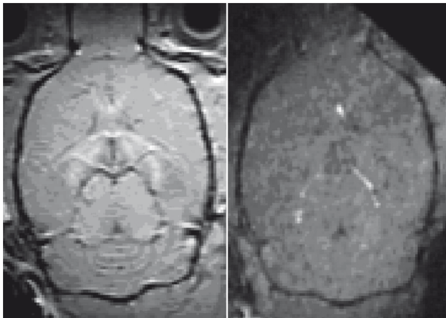
Fig. 3 A MRI of the mouse brain in vivo using a high temperature superconducting radiofrequency coil ( left ) and a conventional copper coil of the same geometry ( right ), both operating at 1.5 T in a clinical scanner. Acquisitions were performed using a gradient-echo sequence. See Poirier-Quinot et al. (2008) for details. Courtesy of Marie Poirier-Quinot, Jean-Christophe Ginefri and Luc Darrasse, Université de Paris Sud – CNRS, Orsay, France
