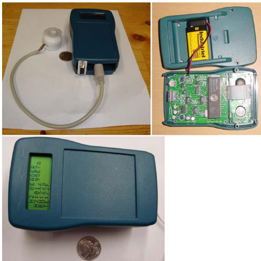
Fig. 3.21 Photos showing packaged sensor with cable connecting sensor to electronics, as well as internal view of sensor electronics [79]
