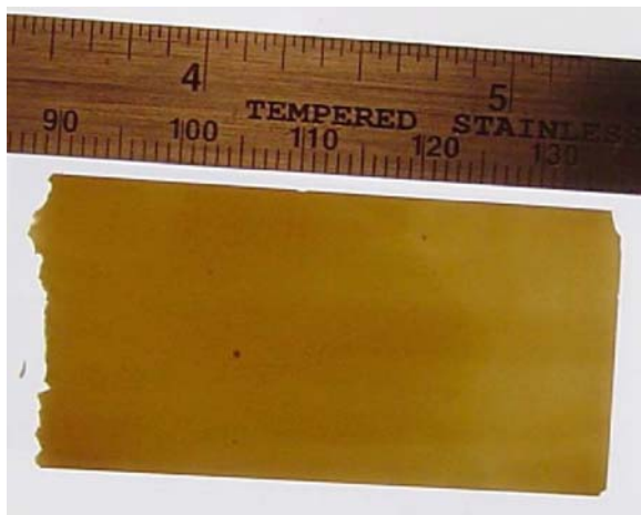
Fig. 1.23 A stable, mechanically robust nanotube array membrane after critical point drying. The 200 \mu\text{m} thick membrane, 120 pore diameter, is about 2.5 cm \times 4.5 cm [115]
