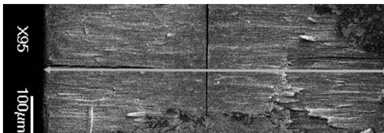
Fig. 1.16 FESEM images of a 720 \mu\text{m} thick membrane synthesized using a fixed 60 V potential for complete, double-sided anodization of a Ti sample after 96 h [54]
