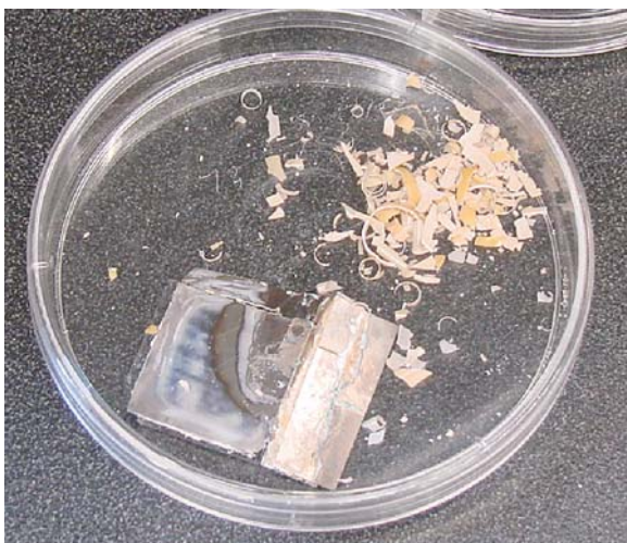
Fig. 1.22 If dried in air the \text{TiO}_2 membrane curls and shatters into shards, as shown above after about 24 h of air drying in air; the diameter of Petri dish is 90 mm [115]
