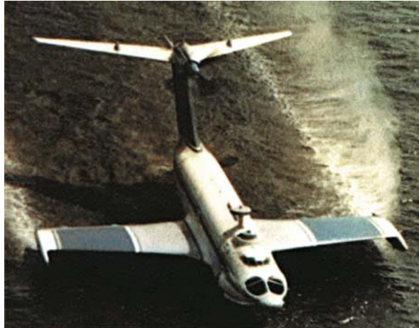
Fig. 11.6 Orlynok showing bow intakes
