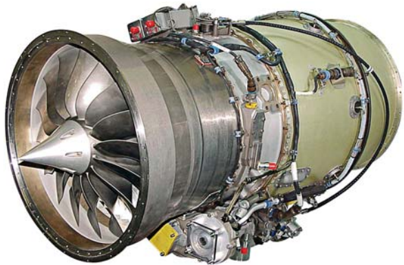
Fig. 11.5 FJ44-2C 2,300 lb thrust fanjet engine
