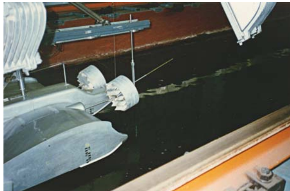
Fig. 7.6 Model test in waves in towing tank
