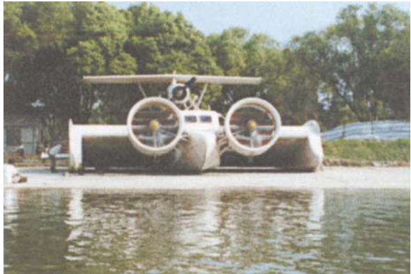
Fig. 4.21 Static hovering test of Swan with people turning it
