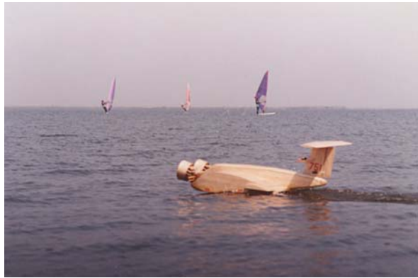
Fig. 3.3 Radio-controlled self-propelled model cushion borne on the lake
