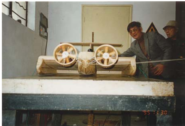
Fig. 4.10 Static hovering experiment of a WIG model on a rigid screen (front view)
