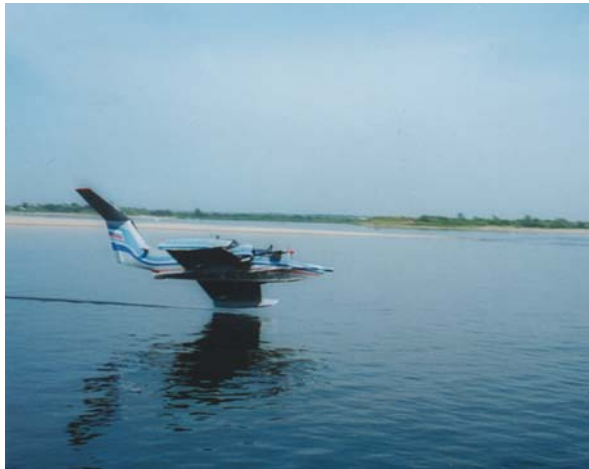
Fig. 3.5 (a) Chinese PARWIG “XTW-I” and (b) “XTW-II” in flying in ground effect
