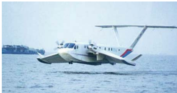
Fig. 2.32 Chinese test PARWIG type “XTW-II”
