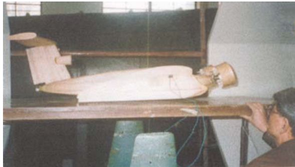
Fig. 4.11 Static hovering experiment of a WIG model on a rigid screen (side view)
