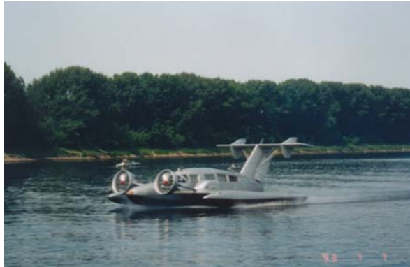
Fig. 2.27 Dynamic air cushion craft (DACC) type “Volga-2”
