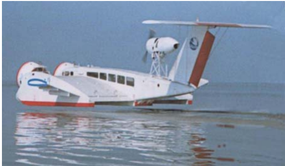
Fig. 7.29 Picture of Swan Mk 2 showing composite wing fences
