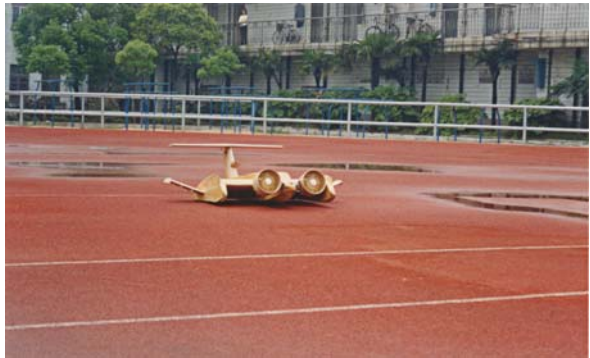
Fig. 4.17 Radio-controlled model DACWIG hovering over land
