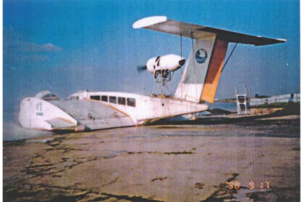
Fig. 4.18 MARIC Swan taking off from the launch ramp on hover
