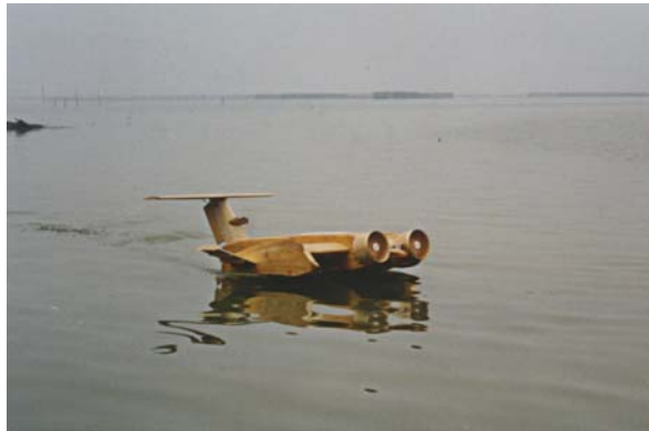
Fig. 7.3 Same model operated in calm water during take-off
