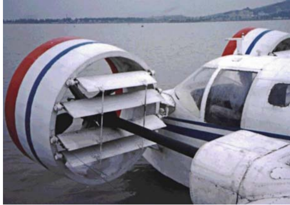
Fig. 12.5 TY-1 propulsor installation
