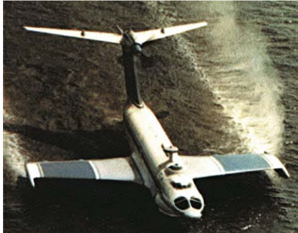
Fig. 11.6 Orlynok showing bow intakes
