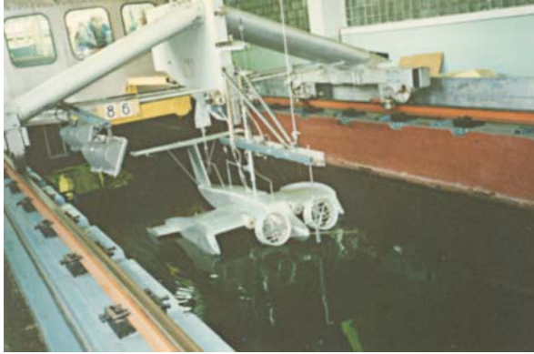
Fig. 7.4 DACWIG model test in towing tank (model suspended before test)
