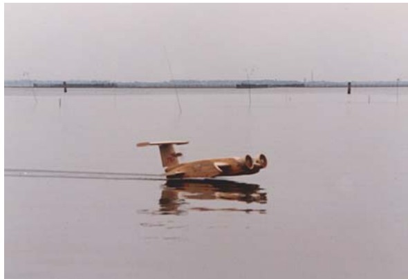
Fig. 3.4 Radio-controlled self-propelled model flying on the lake
