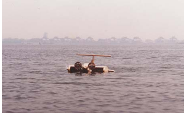
Fig. 3.2 Radio-controlled model operating hull borne on the lake
