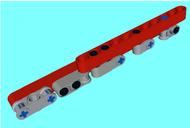
Figure 1-24. Once the Cross Blocks are in place, a Beam or other LEGO Technic pieces can be secured at 90 degrees
