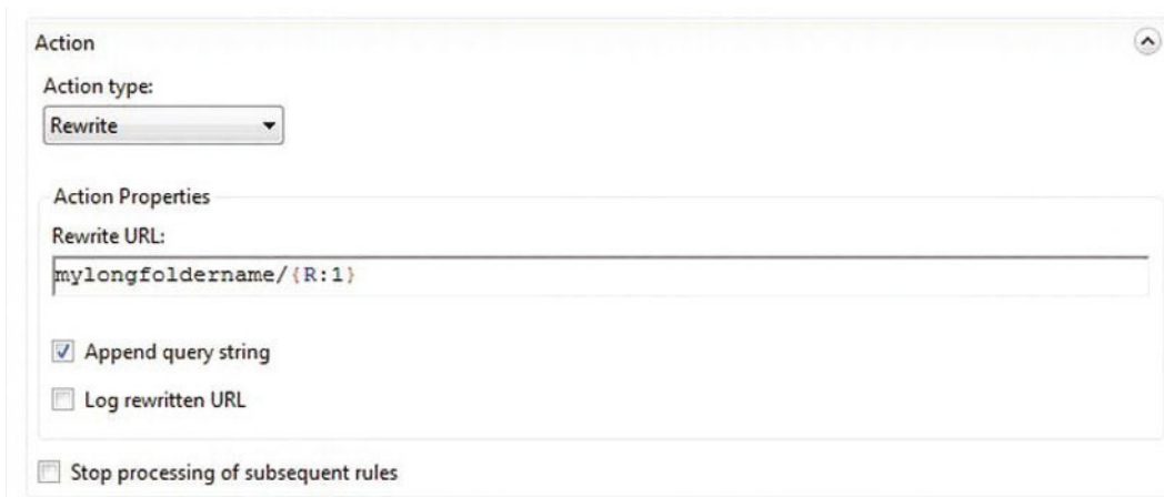
Figure 4-14. Entering the rewrite URL using a capture group from the regular expression
