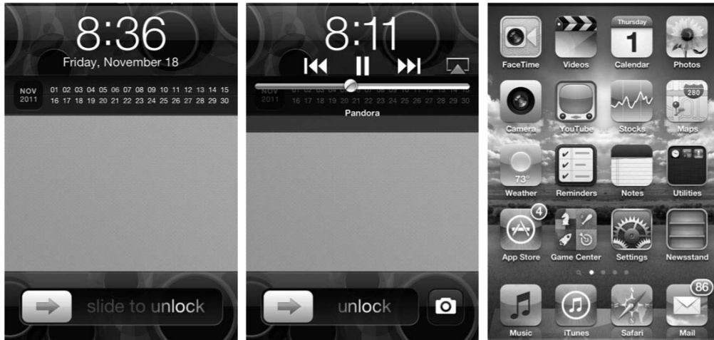
Figure 1-5. Slide to Unlock, Quick Camera and Media Access and your Home screen.
