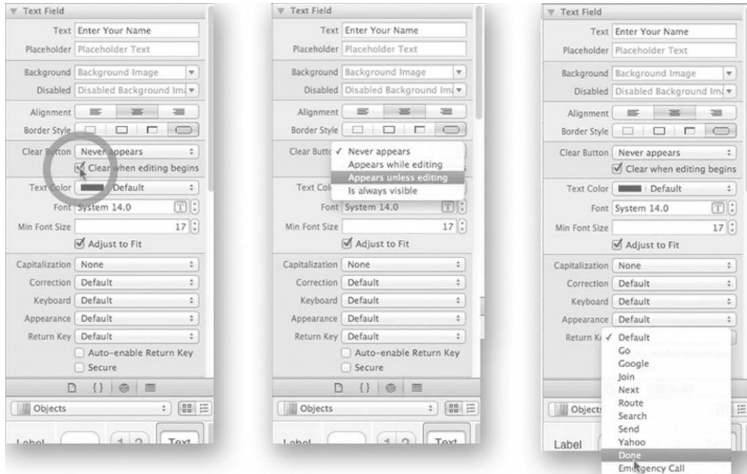
Figure 3-12. The three steps that ensure that the text in the Text Field object clears the instant the user activates the field. Also, note that a clear button icon is in the field, and “Done” appears on the Return Key (see Figure 3-32)
