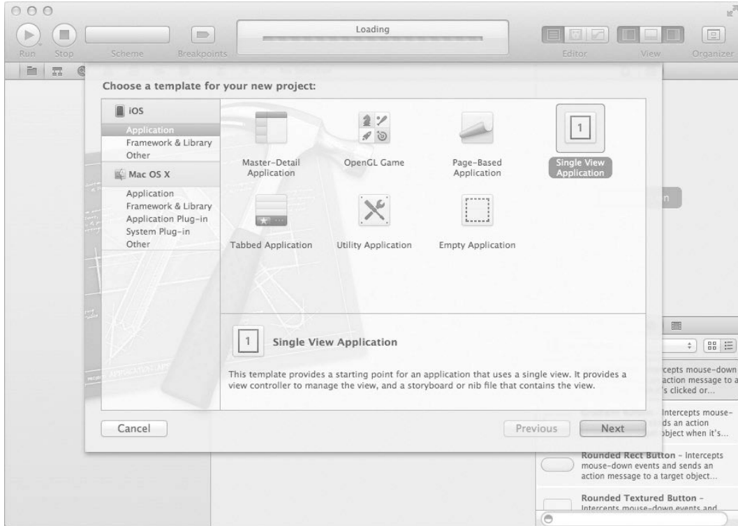
Figure 4-5. Enter \text{⌘} \uparrow N and select Single View Application from the New Project window.
