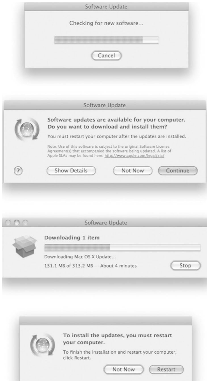
Figure 1–5. Top - Checking for new software; 2nd from the top - Select the option to download the new software; 2nd from the bottom - Wait for your new software to download; Bottom – Select “Restart” to have your Mac properly install the new software.
