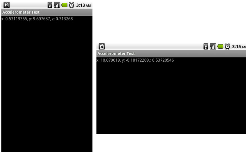
Figure 4–9. Accelerometer axis values in portrait mode (left) and landscape mode (right) when the device is held perpendicular to the ground
