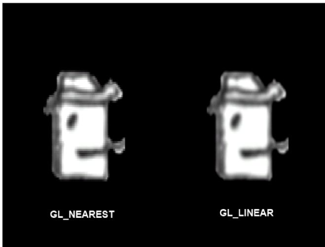
Figure 7-12. GL10.GL_NEAREST vs. GL10.GL_LINEAR. The first filter type makes for a pixelated look; the second one smoothes things out a little.
