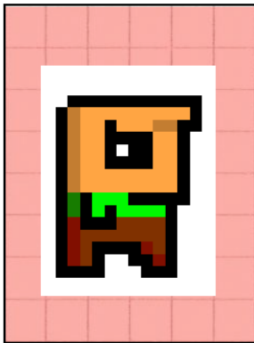
Figure 3–25. Compositing the background and Bob into the framebuffer (not what we wanted)
