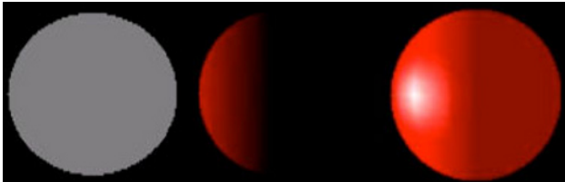
Figure 11–3. Different material/light types. Left: ambient only. Middle: diffuse only. Right: ambient and diffuse with specular highlight.
