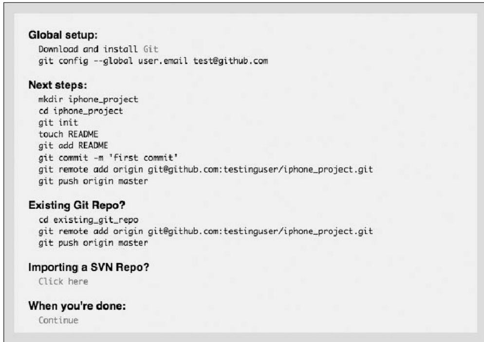
Figure 4-7. Instructions for a new repository
