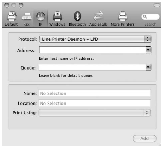
Figure 6-23. Adding a networked printer to a Mac client machine via the System Preferences/Print & Fax tool
