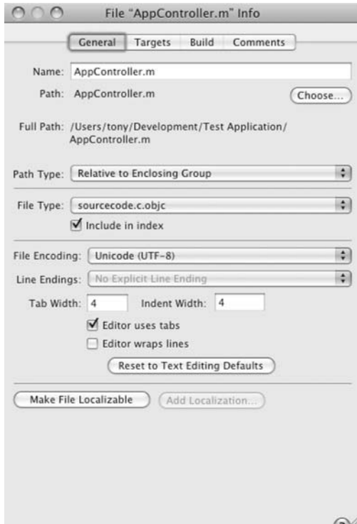
Figure 8-12. Information about the current file available from the main Xcode interface window
