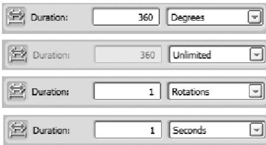
Figure 4-8. There are four options for the Duration section of a MOVE block.
