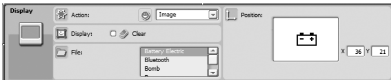
Figure 3-8. Choose an image from the File section to place on the LCD.
