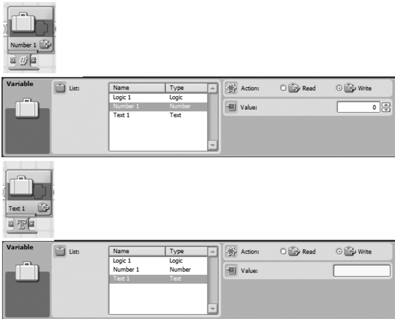
Figure 18-6. The VARIABLE block with Write selected for the Number 1 and Text 1 variables
