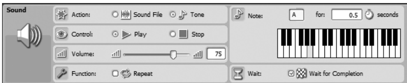
Figure 6-3. The Tone option allows you to specify tones from the Note section.
