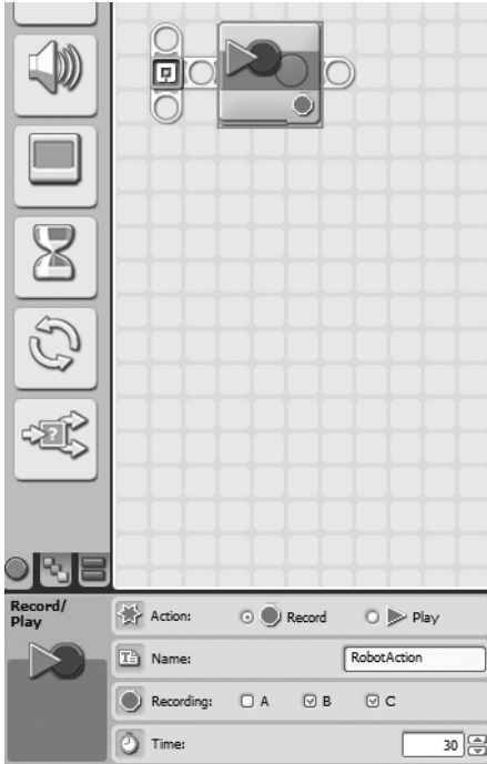
Figure 5-2. Start recording a bot's movements with the RECORD/PLAY block.
