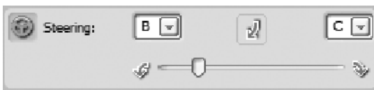
Figure 4-6. The MOVE block's Steering control in the configuration panel
