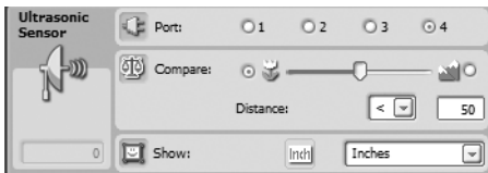
Figure 9-8. The Ultrasonic sensor’s configuration panel
