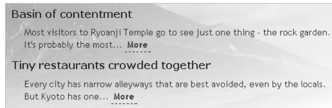
Figure 14-2. Two lines of PHP code produce a more elegant result by ending the extract on a complete word.
