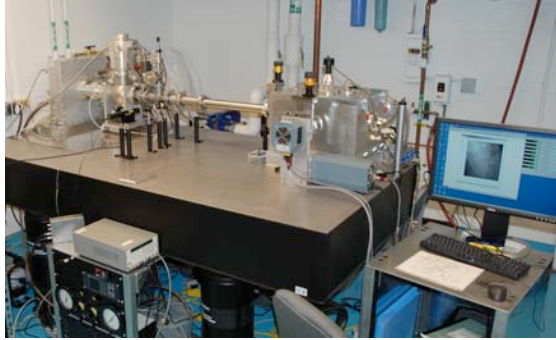
Fig. 1 a) Picture of the EUV microscope. The laser unit on the left is connected through standard vacuum fittings to the microscope chamber on the right. The entire system fits on a small optical table.
