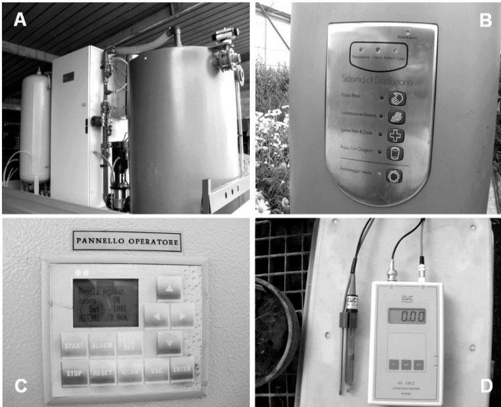
Figure 12. Ozone generators. Mobile ozone generator for field applications (A); for smaller applications (B); panel control to adjust ozone concentration (C) and ozone meter to control ozone concentration in ozonated water (D).
