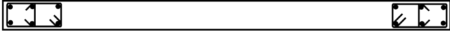
Fig. 5.5 Hoops around boundary elements and cross-ties engaging vertical bars in “large lightly reinforced wall”
