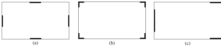
Fig. 2.2 Arrangement of walls in plan: (a) preferable; (b) restraining the floors and difficult to provide foundation at the corners; (c) vulnerable in case of failure of an individual wall
