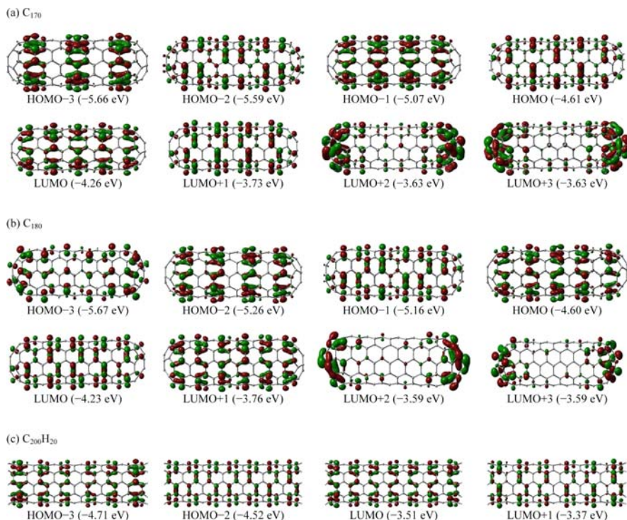
Figure 16-2. The frontier molecular orbitals of (a) the nanorod C_{170} with D_{5h} symmetry, (b) the nanorod C_{180} with D_{5d} symmetry, and (c) the open-end (5,5) SWCNT segment C_{200}H_{20} . HOMO- n ( p eV) is the n th orbital below the HOMO with orbital energy p eV. LUMO+ m ( q eV) is the m th orbital above the LUMO with orbital energy q eV. This figure is adopted from Refs. [94, 180]
