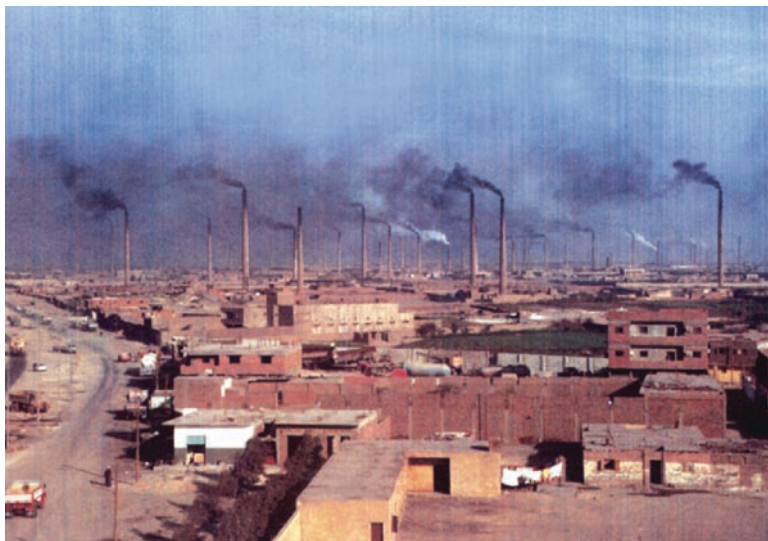
Fig. 3 Cairo/Tebbin South Area: Black plumes are from Mazout burning brick kilns; white plumes are from lead smelters
