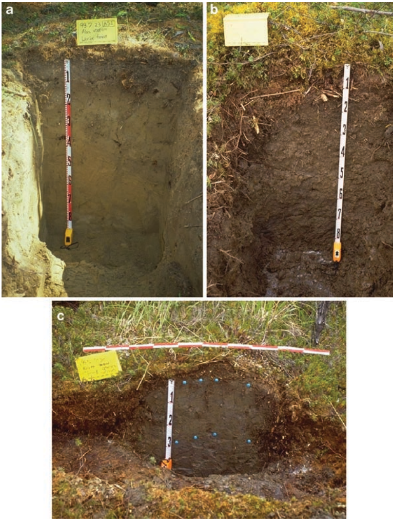
Fig. 8.1 Typical soil profiles under larch forests; (a) in Yakutian basin, Northeastern Siberia (62° 09'N, 130° 38'E), (b) in Central Siberia (64° 19'N, 100° 14'E), and (c) earth hummock mound soil in forest tundra of Kolyma Lowland (68° 41'N, 160° 17'E). Profile (a) had light-colored sandy texture in the active layer. On the other hand, profile (b) had high rock fragment ratio in the active layer with loamy and/or clay loamy texture. In this profile (b), ice-filled cracks emerged at the bottom of the profile. The cross-section of earth hummock mound (c) showed thin A horizon (indicated by white small pins) and bowl-shaped subsoil with diffuse gley mottling (Photos: Y. Matsuura)
