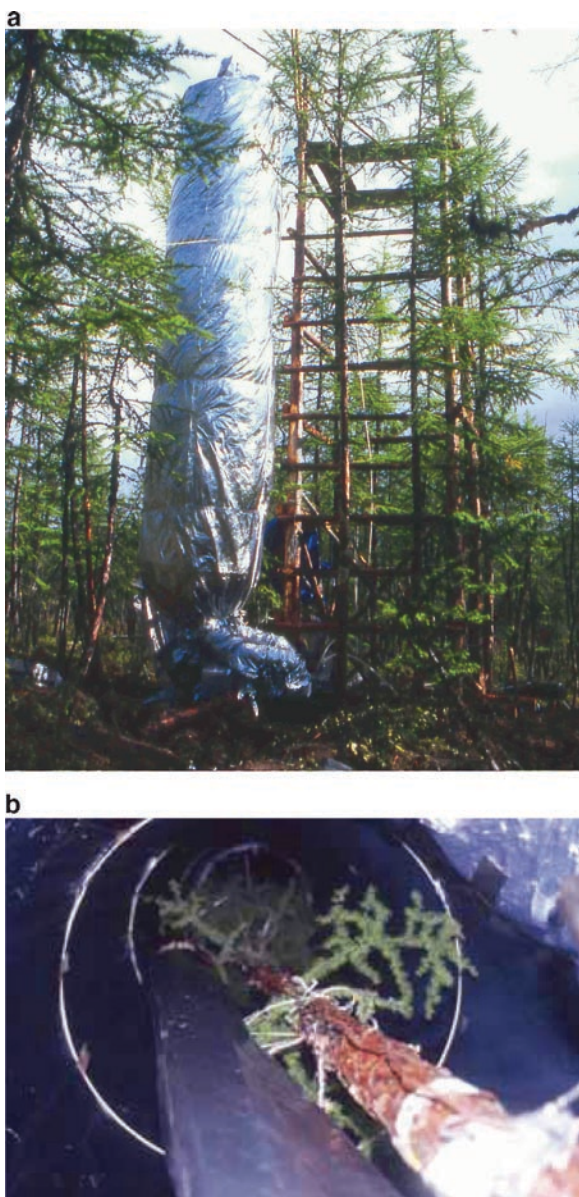
Fig. 15.1 A chamber enclosing a standing L. gmelinii tree (No.2). (a) The chamber was hung from a mast system set at the top of a wooden tower. (b) Inside view of a chamber. Volume, length, and diameter of the chamber were about 9 m 3 , 8 m, and 1.2 m, respectively (photo: Mori)
