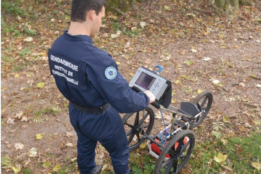
Fig. 13.2 Use of Ground-Penetrating Radar (GPR) to locate illegal graves (photography, IRCGN, France)
