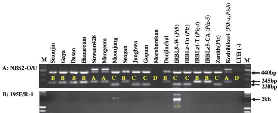
Fig. 1 PCR profiles from genomic DNA amplified by two dominant primers for NSB2-Pi9 (Qu et al. 2006). (A) The PCR products that produced using NBS2-O/U primer set were digested by the restriction enzyme Hinf I and classified into four types, type A of 500-460-240 bp bands, type B of 460-240 bp bands, type C of 460-220 bp bands, and type D of null band, respectively. (B) 195F-1/R-1 primer for NSB2-Pi9 candidate gene produced the positive band for IRBL9-W
