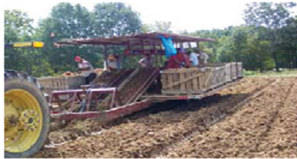
Plate 24 Sweetpotato harvest (2-row mechanical chain harvester) (Courtesy of Tara Smith, Louisiana State University Agricultural Center) (See also Plate 14.11 on page 313)
