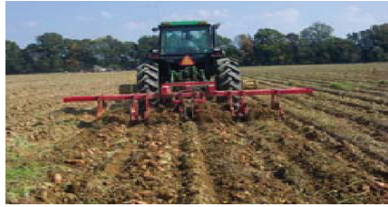
Plate 26 Sweetpotato harvest (shaker harvester method) (Courtesy of Tara Smith, Louisiana State University Agricultural Center) (See also Plate 14.13 on page 314)
