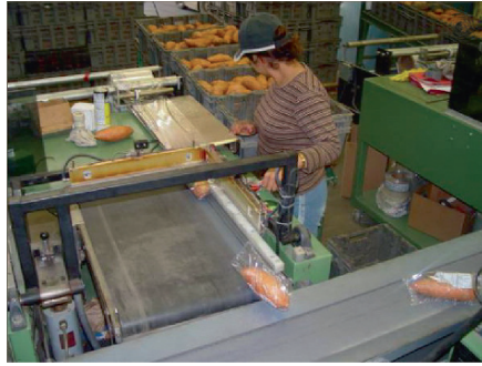
Plate 13 Cello-wrapping of sweetpotatoes on grading line at grower-shipper packing shed in Columbus County, North Carolina (See also Plate 13.4 on page 281)
