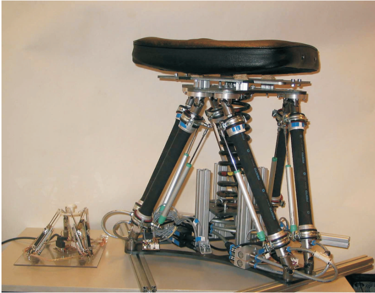
Fig. 1 Photo of the system. The left side of the photo shows the joystick, while the right side is the pneumatically driven hexapod.
