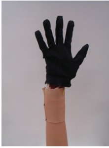
Fig. 11 Five-fingered robot hand using pneumatic actuator
