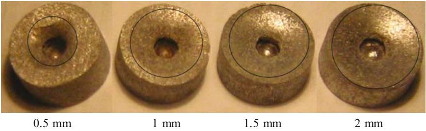
Fig. 6 Top surfaces of Foam I samples after indentation with discs of different thicknesses, before the discs were penetrated. The plastic deformation areas are indicated by circles
